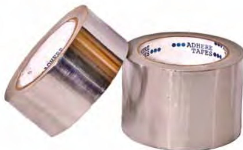
A 0.03MM (NOMINAL THICKNESS) ALUMINIUM FOIL , COATED ONE SIDE WITH GLUE, ACRYLIC, PRESSURE SENSITIVE ADHESIVE, TEMPERATURE RESISTANT, BACKED WITH A STRONG POLYTHENE COATED RELEASE PAPER.
