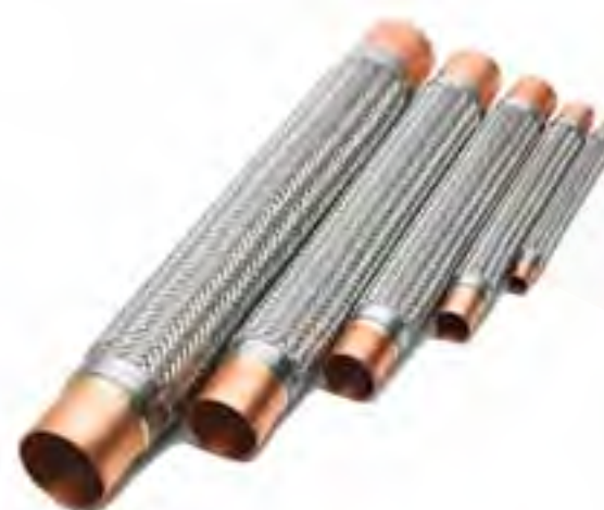
VAF-1 THRU 11 FLEXIBLE TUBING : CORRUGATED BRASS, WIRE BRAID: BRONZ, FERRULE: COPPER, TUBE END: COPPER VAF-82 THRU 87 FLEXIBLE TUBING : CORRUGATED TYPE 321 STAINLESS STEEL, WIRE BRAID: TYPE 304 STAINLESS STEEL, FERRULE: TYPE 30D STAINLESS STEEL, TUBE END: COPPER
